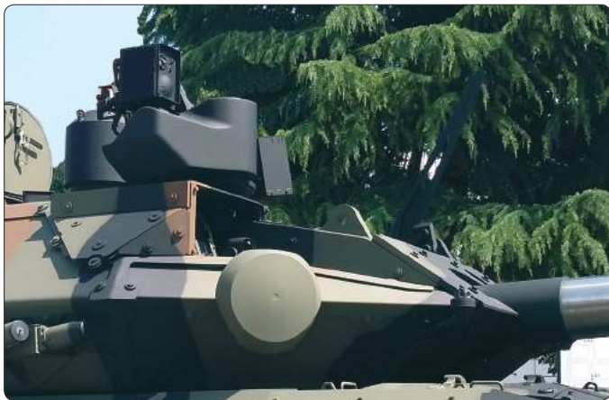
A close-up picture of the Centauro II turret; it is fitted with a Hitrole Light RCWS, here without gun, the round antenna in the foreground being that of the jammer. (CIO)
